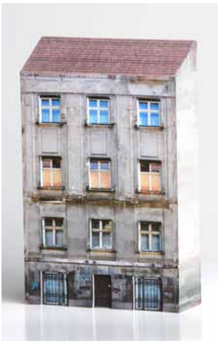
Fig. 9 The Mcor IRIS prints in more than one million colours simultaneously (CMYK, including black), delivering truly photorealistic 3D printed models.
